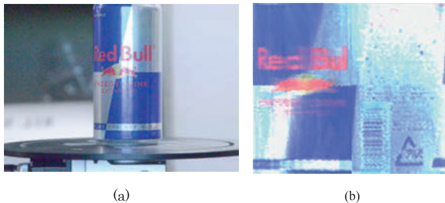
Figure 9 Result of SVBRDF measurement by using aluminum can with multiple texture, (a) Real object, (b) diffuse albedo map.
