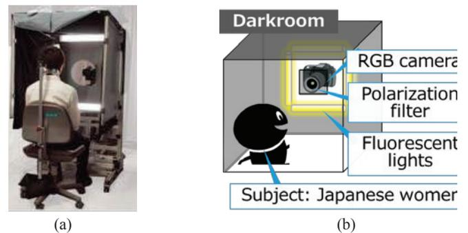
Figure 3 The experimental setup: (a) appearance of the imaging system and (b) overview of the imaging system.
