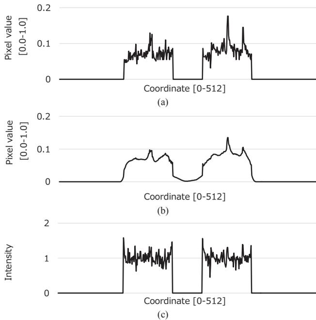
Figure 9 Proposed method as a one-dimensional signal: (a) original signal, a line of surface reflection shown in Figure 8 (a) in 400 rows, (b) smoothed signal in any parameter, (c) a divided signal from (a) to (b).
