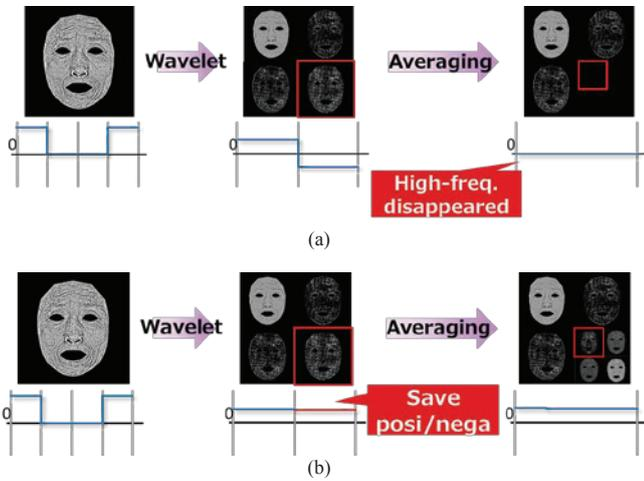
Figure 12 Two-dimensional discrete wavelet transform of high-frequency components:
