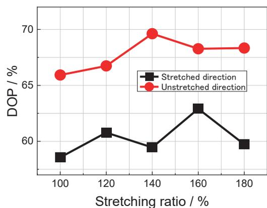
Fig. 11 Degree of polarization of Nafion+CY at each stretching ratio.
