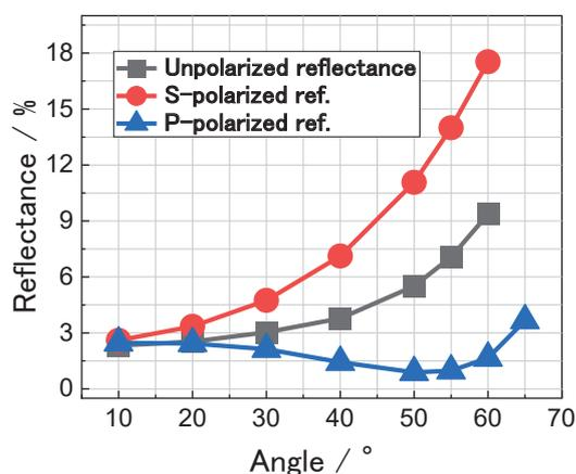
Fig. 5 Fresnel reflectance of Nafion+CV at the wavelength of 540 nm for each angle.
