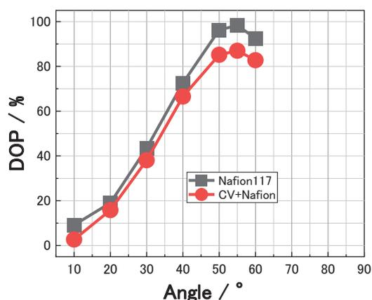
Fig. 6. Degree of polarization of Nafion+CV and Nafion117 sheet at each angle.
