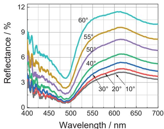
Fig. 4 Specular reflectance spectra of Nafion+CV at each angle.
