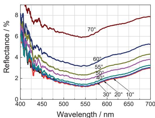
Fig. 9 Specular reflectance spectra of Nafion+CY at each angle.
