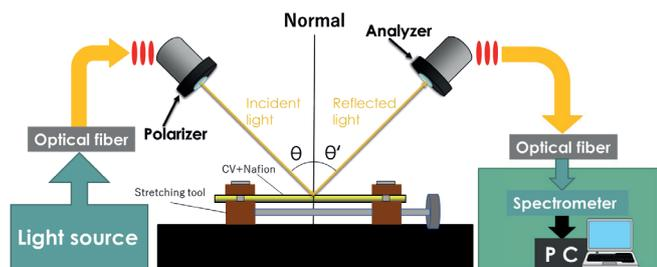
Fig. 2 Schematic diagram of reflectance measurement.
