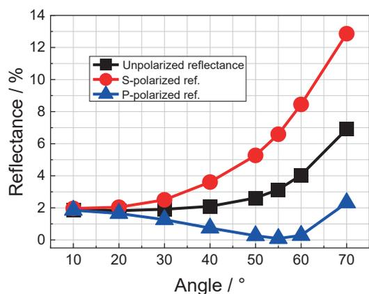
Fig. 10 Fresnel reflectance of Nafion+CY at the wavelength of 600 nm for each angle.
