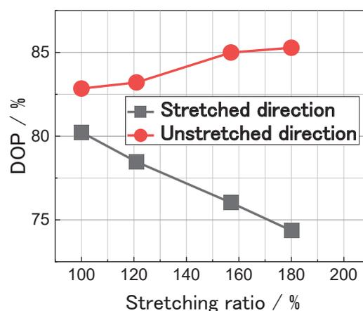
Fig. 7. Degree of polarization of Nafion+CV at each stretching ratio.
